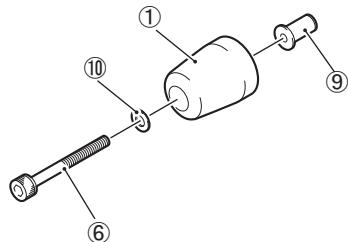
2. Install the Rear Axle Slider (R) ① to the motorcycle.
