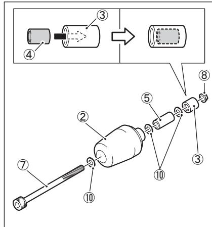
6. Install the Rear Axle Slider (L) ② to the motorcycle.
